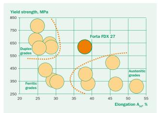
Figure 2. Elongation versus yield strength for different types of stainless steels. Typical values for cold rolled coil and sheet.
