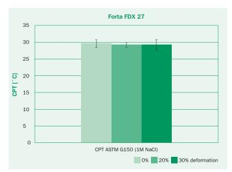
Figure 3. The effect of tensile deformation on the critical pitting temperature (CPT) for Forta FDX 27. Tests were carried out according to ASTM G150 in 1M NaCl. The error bars indicate the standard deviation [1].
