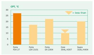
Figure 4. Typical critical pitting corrosion temperatures (CPT) in 1M NaCl measured according to ASTM G150 by using the Avesta Cell. Test surfaces wet ground to P320 mesh. CPT varies with product form and surface finish.
